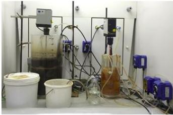
BIO-CHEM-BIO scheme has been successfully applied for MLL in pilot scale. The removal efficiency was even **higher** compared to the lab-scale study.
